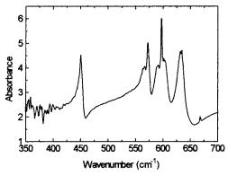
Figure 12. IR spectrum of KLaP<sub>2</sub>S<sub>6</sub>.
