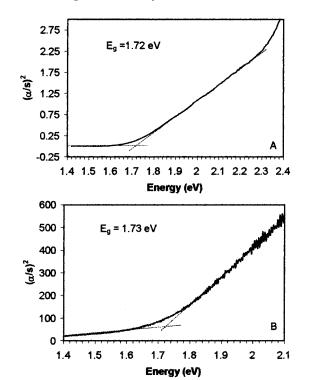
Figure 14. Optical band gap spectra for (A) K<sub>4</sub>Eu(PS<sub>4</sub>)<sub>2</sub> and (B) KEuPS<sub>4</sub>.
