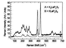
Figure 11. Raman spectra of  $KLaP_2S_6$  and  $K_2La(P_2S_6)_{1/2}(PS_4)$ .
