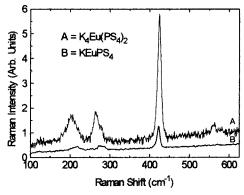
Figure 13. Raman spectra of K<sub>4</sub>Eu(PS<sub>4</sub>)<sub>2</sub> and KEuPS<sub>4</sub>.
